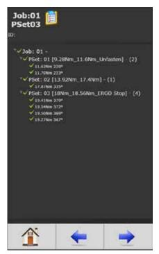
Adding and editing Parameter Sets (256) and Jobs (99) is easy and intuitive in the parameter set up function.
