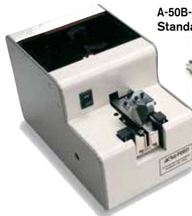
A-50BRBT-4 Compact Robotic Screw Presenter
