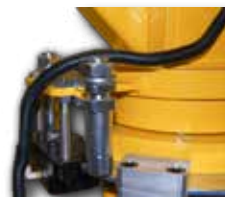
Parking brake and main rotation stops
