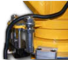
Parking brake and main rotation stops
