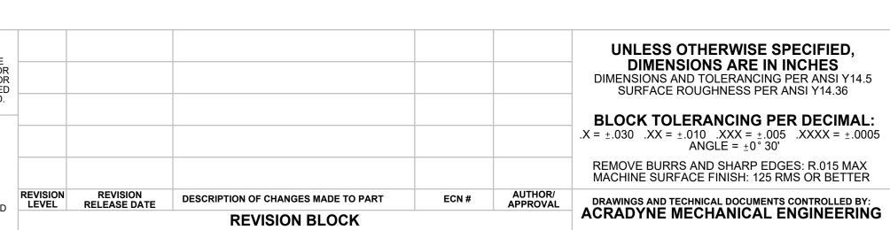
UNLESS OTHERWISE SPECIFIED, DIMENSIONS ARE IN INCHES DIMENSIONS AND TOLERANCING PER ANSI Y14.5 SURFACE ROUGHNESS PER ANSI Y14.36
