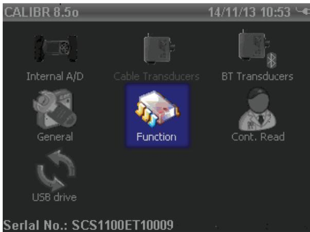
Press OK button to confirm EasyTouch will display the " Calibration menu" window. Press "Function" icon
