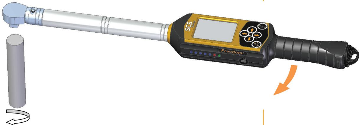
To compensate the extension twist, user need to measure the extension twist degrees on maximum torque tightening
