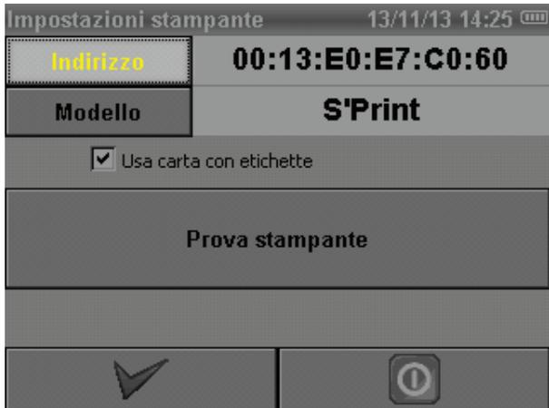
Push "**address**" button and EasyTouch will automatically search the S'print – BT printer.
