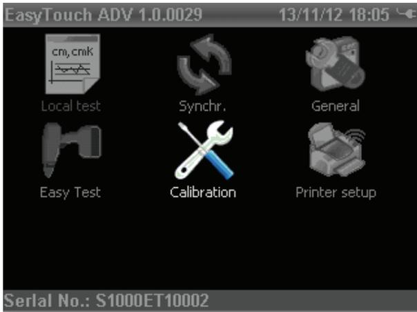
Enter into "Calibration" setup by pressing "calibration" icon. A new window will be displayed and ET will require to enter the password "1247" to proceed. See below image.
