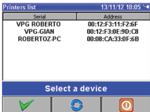
After few seconds EasyTouch will display the BT tools list. Select S' print BT printer and press "confirm" button. Push "update" button, if the user wants to research the printer. Push "Abort" to exit without saving.
