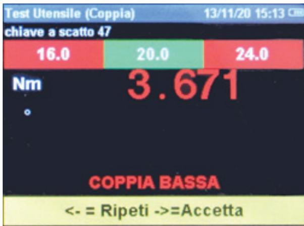
The test has a negative result, if the torque is too low and under the minimum tolerance. In this case the result will be displayed in red color. When the test has a negative result, ET provides the reason by displaying a message.
