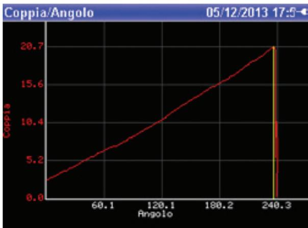
Torque/Angle chart example for a “power tool” test.
