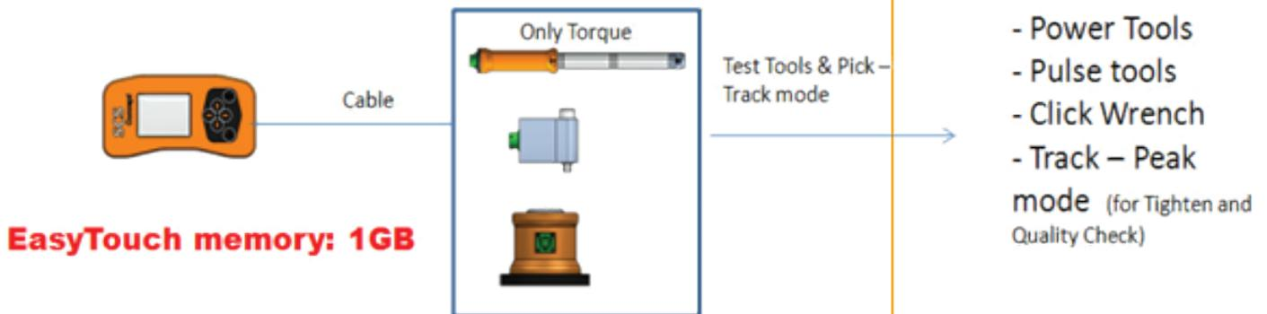
EasyTouch is a data collector designed to perform tests on production line or laboratories by connecting torque or torque/angle transducers.
