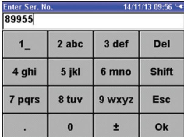
ET will now ask to confirm the transducer serial number written in the transducer memory (in the example 89955). Press OK on ET's keyboard to continue.
