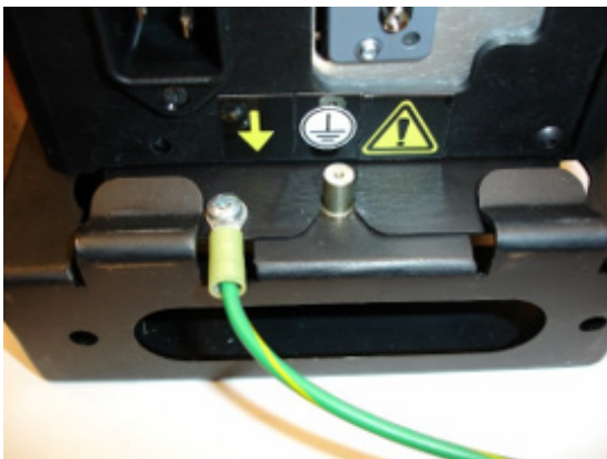
Figure 1 — Secondary Protective Earth Attachment
