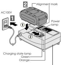
Slide loading type Lithium-ion rapid charger AC100V (225VA) 50/60Hz (with 2-pin plug) Weight: ~ 0.9 kg Service temperature 0°~40° Use dedicated power plug only.
