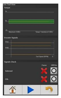
Shows a live view of tool transducer in volts. Voltage will be approximately 0 volts when tool is at rest and torque is zero. During a rundown, the tool transducer voltage increases as torque increases.
