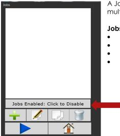
A Job is a collection of PSets which can be run when performing multiple fastening operations on a single application.
