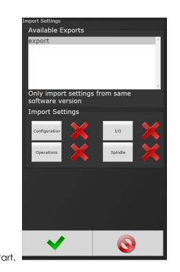
Import settings that were exported from another controller via a USB flash drive. Use this to quickly apply the same settings across several controllers. For example, it is common to have multiple controllers with the same IO configuration. Set up one controller with the correct IO configuration and export the controller from Advanced->Export Controller. Now the IO settings can be imported using this screen.
