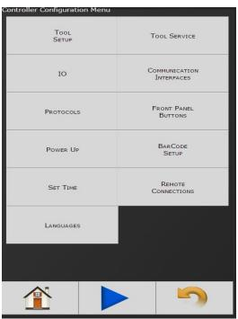
The controller menu is where all of the settings for the IAC controller are configured. All of the different configuration capabilities are explained below.
