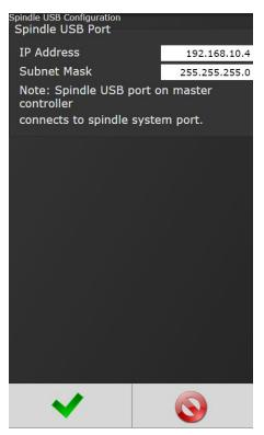
This can be used to set up a 2 spindle network through the USB port
