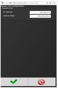
IP Address: The IP address of controller's System Port (Default is 192.168.1.4) Subnet Mask: The Subnet Mask of controller's System Port.
