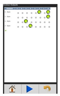
Click on 😑 to make changes on an individual Element or return to the Output Configuration screen.
