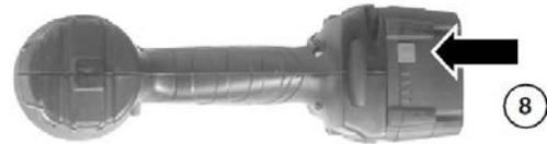
Push button (8) on the battery pack and check the charge status. If the battery pack is almost empty, it must be recharged. Replace the battery pack on the power tool.
