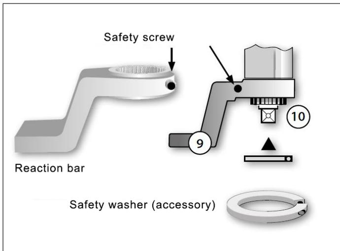
For reaction bars without safety lock, a safety washer is available as an accessory. This washer prevents a loosening of the reaction bar and can be pushed over the gear cogs and screwed tight.
