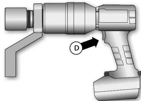
**Switch on:** Push and hold button (D). The electronic control system will ensure a soft start.
