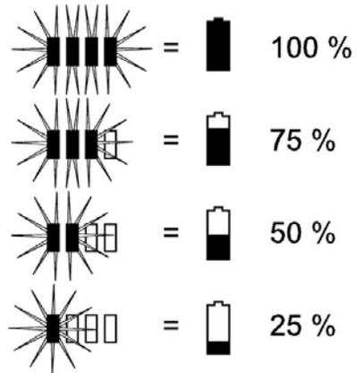
If one of the LEDs flashes, the battery pack is almost empty. The electronic circuitry protects the battery pack against damage due to complete discharge. Replace battery back on the power tool. Recharge battery pack.
