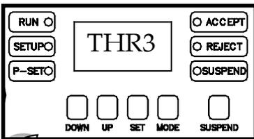
desired threshold abbreviation is in view (THR1, THR2, or THR3). While the threshold abbreviation is on the display, press the SET button.
