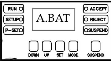
Once at this display, the SET key can be pressed in order to view or program the batch setting. After the SET key has been pressed, the display will show the current amount programmed into the batch. Also, the digit in the 100's column will be flashing. The UP and DOWN keys can be used in order to change the value of the flashing digit.
