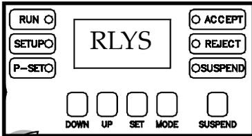
Within the AIM Tightening Monitor there are three relays that signal batch accept, cycle accept and reject. These relays can be set to be latching or momentary.
