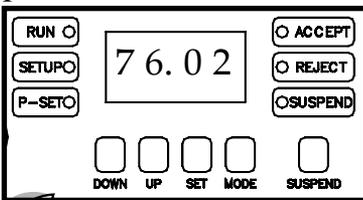
The left two digits on the four digit display will show the analog value for channel 1. The analog value for channel 2 will appear on the right two digits of the display in this mode.
