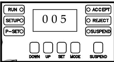
Pressing SET again will lock in the value for the flashing digit and cause the next digit to the right to begin flashing. This process may be repeated until the desired value is programmed into the batch.
