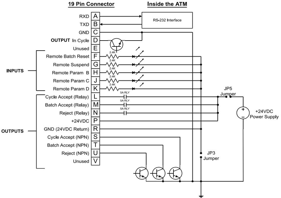
JP3 and JP5 on this diagram can be found on the back-board (CE2891) inside the AIM Tightening Monitor.
