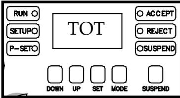
The total number of completed batches is one of the values that can be viewed in the monitor mode. In order to clear this value for any given
