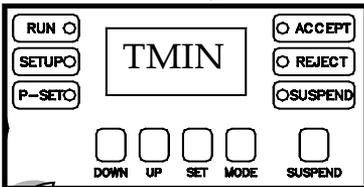
PROG position and press the MODE button until the desired abbreviation is in view (TMIN, TMAX, or TCLU).
