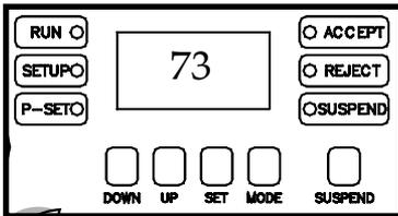
old will appear on the display with the left most digit flashing. The UP and DOWN buttons may be employed to adjust the flashing digit. Once
