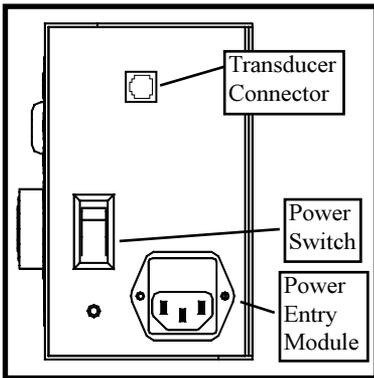
The power entry module can be set to accept either 110VAC or 220VAC for its power. This setting is visible through a small window on the power entry module. **Be certain that the appropriate voltage is selected prior to applying power to the unit!**
