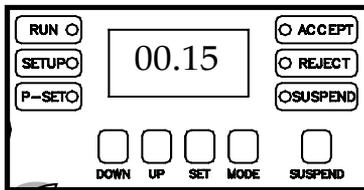
be visible on the display and the left most digit will be flashing. The UP and DOWN buttons may be pressed in order to edit the flashing digit
