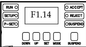
To determine the firmware versions that are running in any given AIM Tightening Monitor, turn the key to PROG and press the MODE button until the display read FX.XX or BX.XX.
