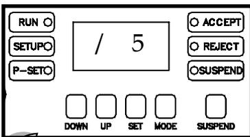
is the current parameter set (A-D). Once the MODE button is released, the display will show the number of fasteners in the batch. The batch can be
