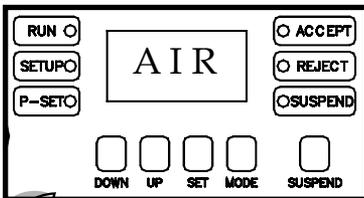
monitor mode. If the MODE button is pressed until the display reads TYPE, when the button is released, the display will give an indication of the
