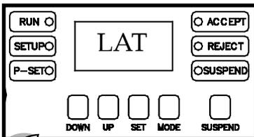
In order to set this value, turn the key to the PROG position and press the MODE key until the display reads RLYS. Once at this display, press the SET button and the display will either read LAT (for latching) or MOM (for momentary).
