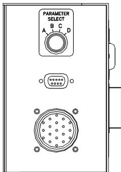
The left side of the unit contains a parameter selection switch, a 9 pin D-SUB connector, and a 19 pin circular I/O connector.
