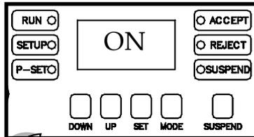
the SET key is pressed the display will either read “DBL BEEP ON” or “DBL BEEP OFF”. Pressing the SET key will allow the user to toggle between these two values.
