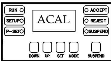
In order to enter AutoCal™, insert the key into the unit and rotate it from LOCK to PROG. As the key reaches the program position, the display on the ATM will read PROG, MENU, and then ACAL.
