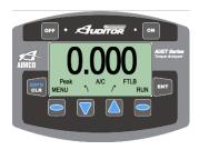
the **LEFT SELECTION BUTTON**, which is directly below the **MENU** text field, would allow the user to access the **MENU** features.
