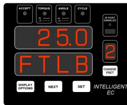
Example: PSET #2, Torque Control Strategy, 25 ft-lb Target
