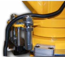
Parking brake and main rotation stops
