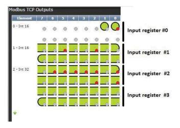
The controller's outputs can also be addressed as coils. The assigned outputs start at coil #16.
