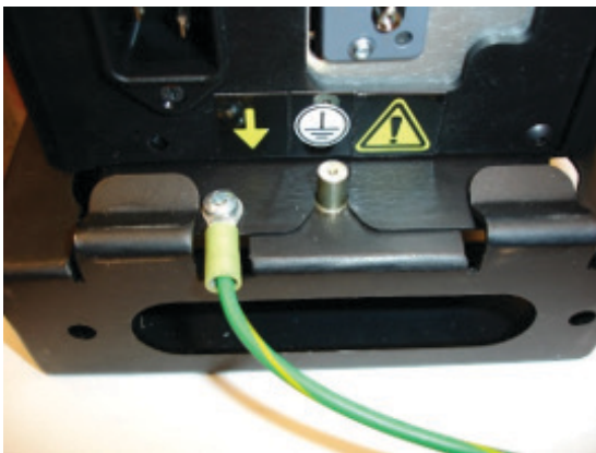
Figure 1 — Redundant Earth Ground Attachment
