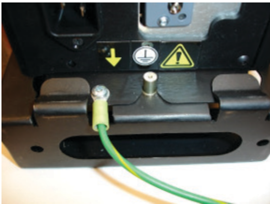
Figure 1 — Redundant Earth Ground Attachment
