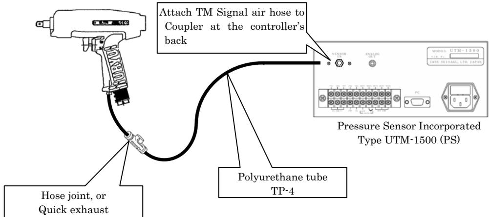
④When using Air-electric Relay
