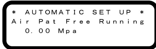
① Run your Tool for 2~3 seconds under no-load, and then release the lever.
