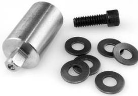
The Joint Kit is made up of a series of **Belleville Washers** that allow the user to pre-configure the joint to match the actual application joint as closely as possible. Each of the **Belleville Washers** is concave in shape. By aligning all the concave curves in the same direction a simulated hard joint is achieved (Fig. B).
