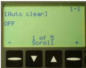
When unit is returned to operational mode, AC will show on the bottom of the display. Because AutoClr is now active, the reading will show for the specified number of seconds and then clear the display. At this point, all readings will clear and be stored automatically into memory.
