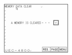
Enter MEMORY DATA screen and a message [A MEMORY IS CLEARED ...  $\boxed{Y}$ ] appears. Touch $\boxed{Y}$ , and UEC starts clearing the memorized data. A message [MEMORY CLEARING...] while UEC is clearing the memorized data, and a message [MEMORY CLEAR END] appears when UEC finishes clearing the memorized data.
