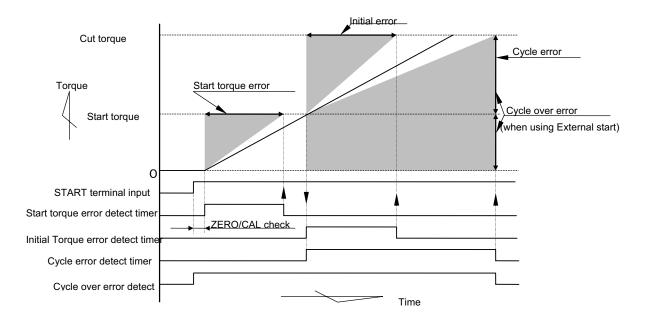
Note) Above is an example of linear torque change curve.
