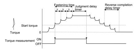
UEC starts torque measurement when detecting the start torque or greater torque, judges the tool is shut off when provides judgment when the fastening time between peak torque (x in a graph) gets longer than the judgment delay timer, and provides judgment.
