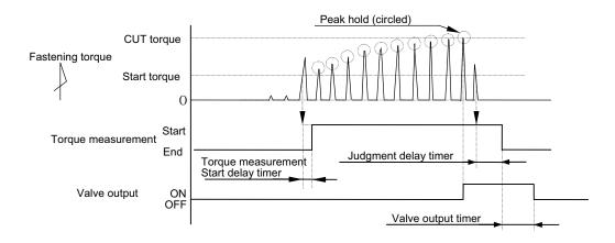
5) T type wrenches Torque and fastening time monitor Control method: 9 UEC monitors torque and fastening time of shut off tools.
