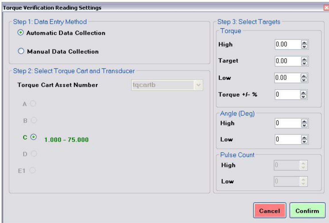
5. The Torque Verification Settings Window will pop up. Select the Transducer port for the appropriate transducer.
