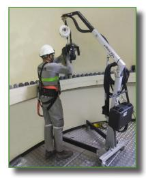
Designed for tool suspension and use, the Lift Assist allows for easy maneuvering and easy handling and of equipment that otherwise would need two operators to position.
