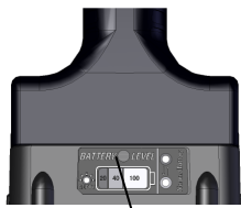
Battery gauge LED
