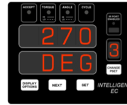
Example: PSET #3, Angle Control Strategy, 270 Degree Target
