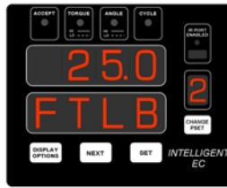
Example: PSET #2, Torque Control Strategy, 25 ft-lb Target
