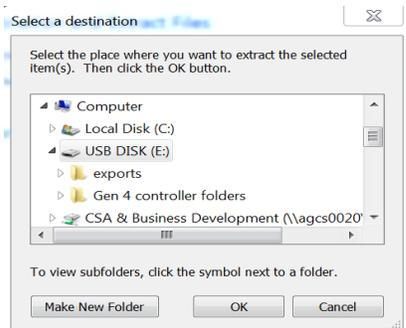
If unable to Import file from USB, check directory structure. The files on the USB drive should be in the following directory structure:
