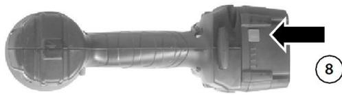
Push button (8) on the battery pack and check the charge status. If the battery pack is almost empty, it must be recharged. Replace the battery pack on the power tool.
